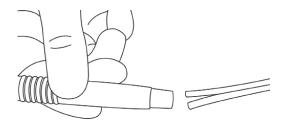
B Push the twin tube all the way through.
