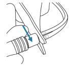
Tilt the key against the body of the handpiece to ease off the twin tube.
