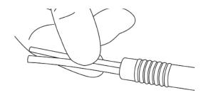
Attach the twin tube to the cutting tip. Make sure the narrow tube is attached to the narrow socket and the wider tube to the wider socket.
