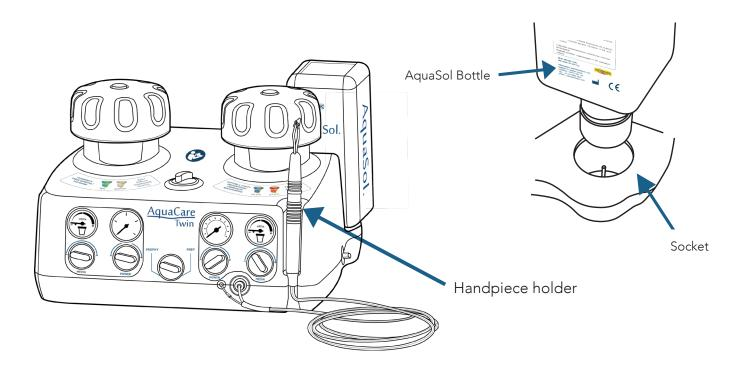
The handpiece holder needs to be cleaned on a regular basis to remove any contamination that may have been transferred from a contaminated handpiece handle. Use a cotton bud soaked with AquaSol to clean the holder.
