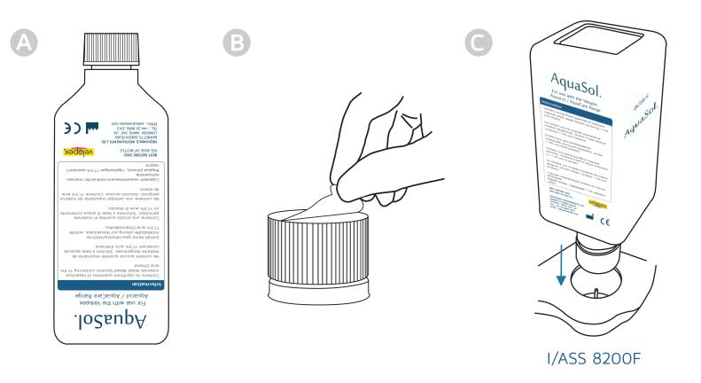
WARNING: The above fluid container is filled with a 17% alcohol solution. This acts as a biostatic solution in order to reduce biological growth within the fluid system. NOTE: Not for human consumption.
